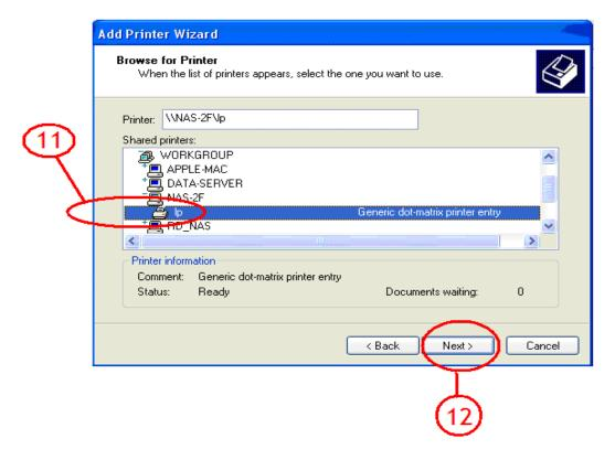
G. Go to Printer wizard and select the printer driver. Click "OK" to complete setup.
