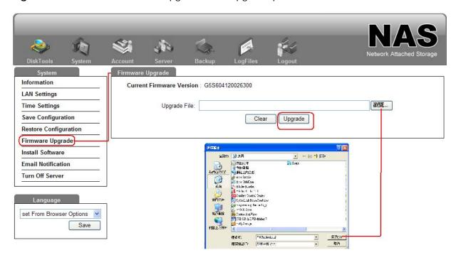
B. Connect the NAS directly to your PC by a network cable, than start update the firmware,
