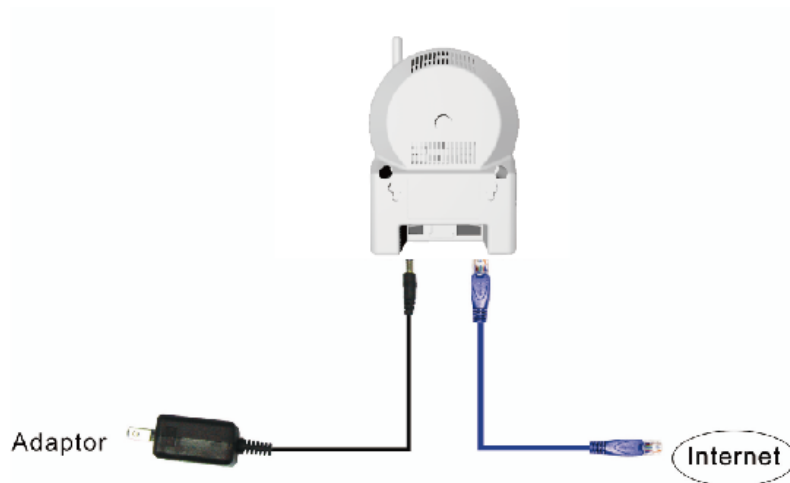
Figure 2-3: IP CAM connection diagram.
